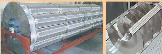
Inside the dryer, the climatization system circulates air throughout the winding cage in opposite direction of screw rotation. Moisture levels are closely controlled by an electronic sensing device that measures the humidity level and activates the moisture extraction process when required. Each rotation of the cage transports the product from one thread to the next inside the Archimedes screw.
