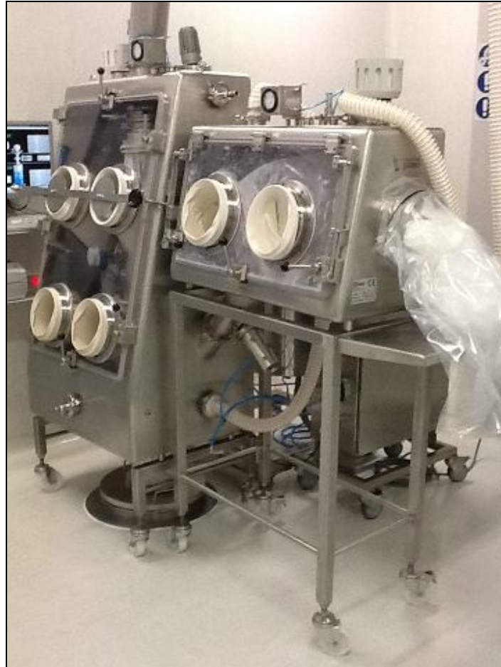
DOUBLE CHAMBER ISOLATOR FOR PRODUCTION SCALE CONE MILL
