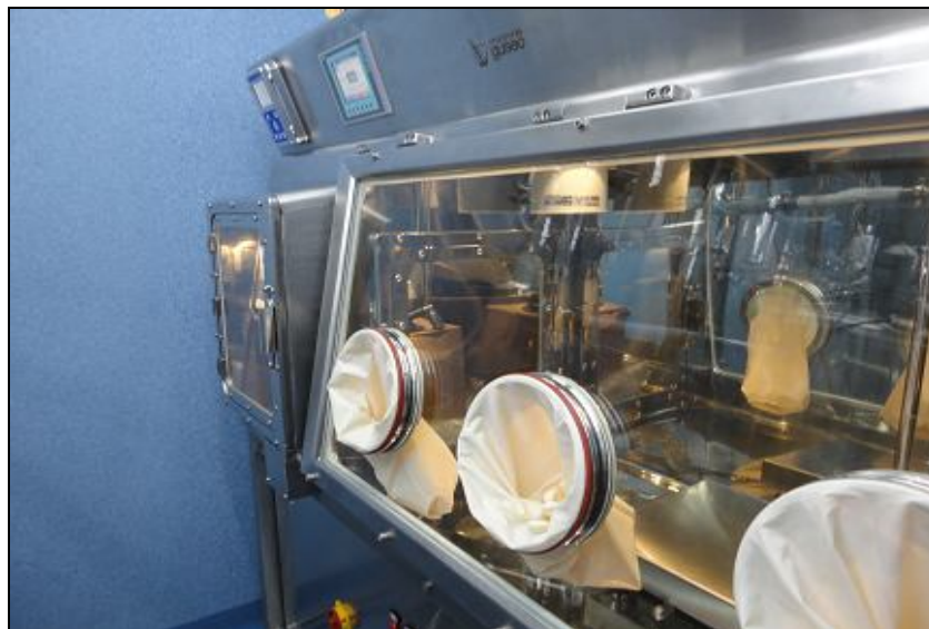
DOUBLE CHAMBER WEIGHING AND DISPENSING ISOLATOR
