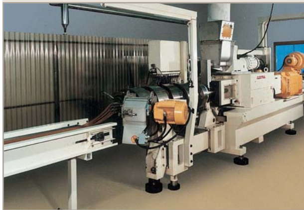
Dense strands of processed grits exit the extruder. After a brief cooling period, the strands are cut into nibs, and flaked to form the finished product.
