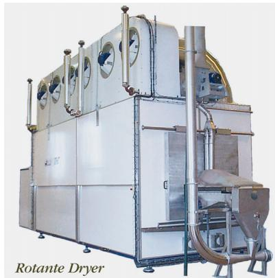
drying sensitive products such as pellets. The product is very gently conveyed within single Archimede's screws positioned around a moving drum, maintaining perfect product integrity. There is no residence
