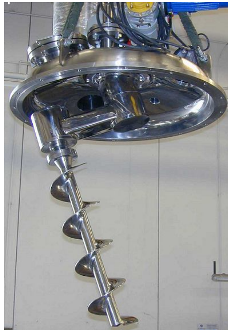
Detail of the upper cover internal part with screw agitator
